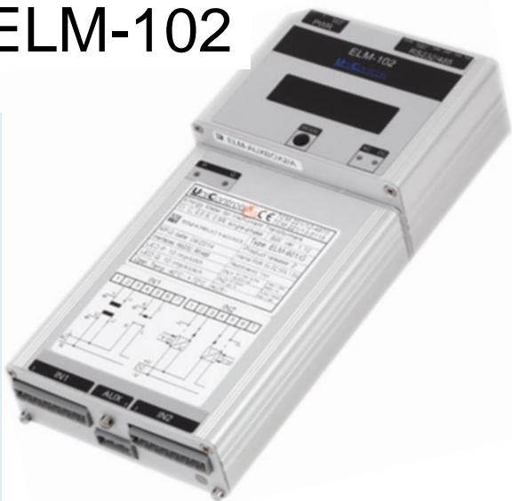
The **ELM-102 energy meter** is designed especially for energy metering onboard electric traction vehicles. It can measure both the DC and AC signals of any existing traction supply system (1.5kV DC, 3kV DC, 15kV/16.7 Hz, 25kV/50Hz). Moreover, it is also suitable for multi-system locomotives using more than one electrification system.
