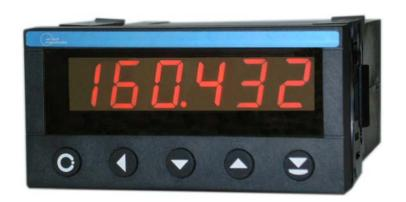
Model OC 7171A-I is a very instrument for time precise integration of analog signals. The heard of the instrument is a programmable counter with input signal conditioner which converts the analog input signal into a precise frequency spectrum. The resulting time integration has very high degree of accuracy and linearity. The momentary value as well as the totalized amount of increments are available at the display and can be selected with the keyboard.
